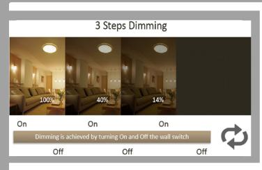
Goldwyn's new 3 Step Switch is a unique way of dimming by just turning ON and OFF the wall switch. The first cycle corresponds to 100% LED brightness followed by the second and third cycle corresponding to 40% and 14% LED brightness respectively. This energy efficient switch also comes with overvoltage protection, open circuit protection, short circuit protection and thermal shutdown.
